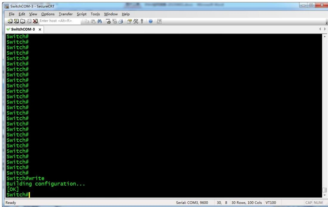
Now, it has successfully saved the current configuration. Core switch will run this configuration for the next startup.
