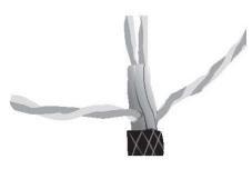
5. Thread the inner pairs (4/5, 3/6) through the wire tray and seat the wires in the proper slots as shown below. Then route the outer pairs on top of the wire tray and seat the wiresas shown. Once the wires are pressed into the slots, trim the excess wires with a pair of flush-cutters.
