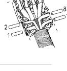
Flip the wire tray upside down and insert it into the connector pressing it firmly into place.
